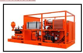
Equipment: Gardner Denver GD-600 Pump, Cummins QSX15 Engine, Allison 4700OFS Trans.
